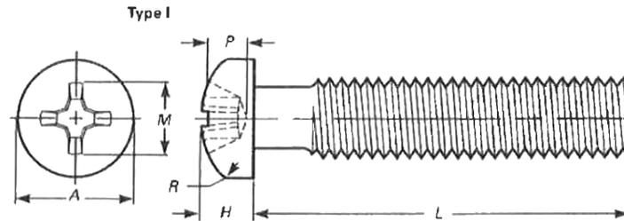
This type of recess has a large center opening, tapered wings, and blunt bottom, with all edges relieved or rounded.
